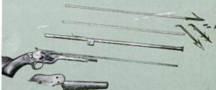
Here are the parts shown disassembled. Third long tube from the top is the flared barrel. Most of the gun is made of stainless steel or bronze to minimize corrosion
